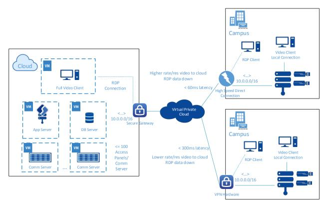
Figure 6. Edge-Based Video Design with Multiple Viewing Options
