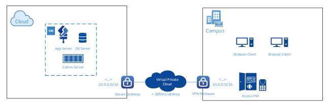
In this scenario, a Virtual Private Cloud is created that extends the campus network to the cloud via secure VPN connections. In the cloud environment, a single VM is instantiated that hosts all of the OnGuard server components. Most cloud providers design redundancy into the physical hosting of their VMs, so this configuration in the cloud is more resilient than a single physical server operating on the campus.
